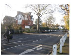
In view of the above and as shown in the drawing overleaf, it is recommended that a 'School Keep Clear' is installed adjacent to the entrance to the James Allen's Preparatory school on Village Way and double yellow lines are installed adjacent to the entrance to the park on Dulwich Village to prevent obstructive parking and ensure inter-visibility between vehicles and pedestrians.
